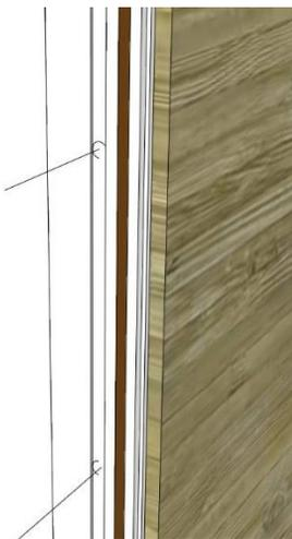
Screw through the Pre Piloted holes with \*100mm\* timber, or Timber to steel screw, depending on the structure build up. If pilot holes aren't present, fix to structure at 250mm from top of door frame, then 450mm centres thereafter. Where possible, keep the door in the frame. Once the frame is fixed to the structure, check that the gap between door and frame is 3mm. This can be tested with a £1 coin. Leaf to FFL must not exceed 10mm
