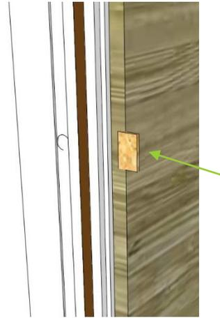
Depending on the gap between wall and structure, wooden packers should be used through which the jambs can be securely attached to the wall. Packers should be used at the position of the hinges if possible.
