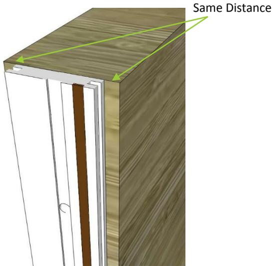
Ensure the Door Liner is centrally located in the aperture to ensure the same distance is either side of the liner
